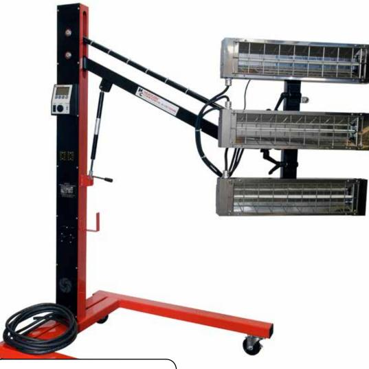
The primary application of the HCS2044 Infrared Curing system is to accelerate the cure of two part resin systems, paint, primers and other coatings.
