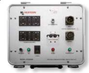
The Network Node Hot Bonder is a high-technology combination of hardware and software used to accomplish large or complex composite
